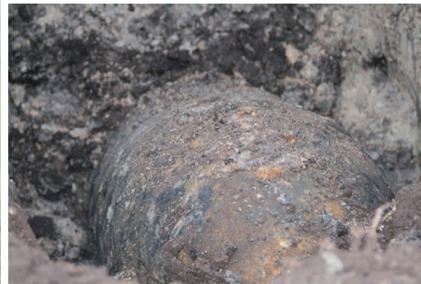
The 1,000 pound medium case, general purpose bomb from Lancaster JB280 exposed to the light of day for the first time since the night of Jan. 2, 1944. These bombs came with one of two types of fuses – an instantaneous contact fuse in the nose and a long-delay (up to 144 hours) fuse in the tail. As the nose of this 1,000-pounder is smooth, this was a long-delay fused bomb. The fusing was clearly damaged in the crash and the bomb was never fused, lying dormant but very much alive for more than 70 years. This type of iron bomb was used for area bombing raids (industrial demolition). Photo by Geert Bos and supplied by Rob Wethly
